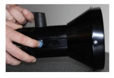
If at any time during operation the black filter glass fitted in front of the UV bulb is broken or damaged in any way, then the torch must be switched off immediately. It must not be used again until a replacement black filter glass is fitted.
