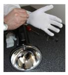
Put on lint free nylon gloves. This will avoid fingerprints contaminating the filer glass during reassembly.
