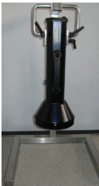
Figure 3: Test set up for measuring the effectiveness of the UV torch at varying distances from the surface
