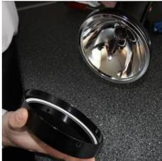
Remove the 4 x M4 screws and washers from the front of the torch.
