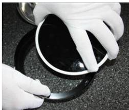
Place the black filter glass back in the filter mounting ring.
