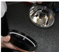
Pull the filter mounting ring off the front of the torch.
