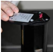
Rotate the battery access door to the fully open position.
