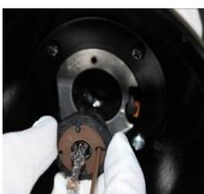
Carefully remove the reflector taking care not to damage the UV bulb.
