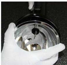
Carefully replace the reflector taking care not to damage the UV bulb.
