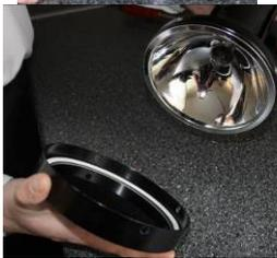
Pull the filter mounting ring off the front of the torch.
