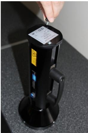
Place on a solid flat surface. Unscrew and remove the thumb wheel on the rear of the torch. Rotate the battery access door to the fully open position.
