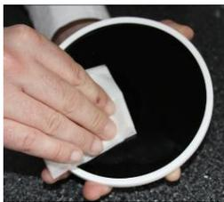
Wipe both surfaces with an alcohol impregnated wipe. Never use any soaps, detergents or abrasive materials.
