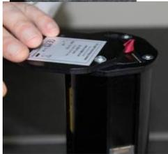
Rotate the battery access door to the fully open position.
