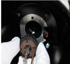
Push new UV bulb into place and rotate clockwise.
