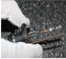
Take a new UV bulb and check for any visible damage. Never use damaged UV bulbs.
