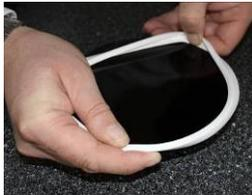
Take a new black filter glass and fit white silicone filter gasket.
