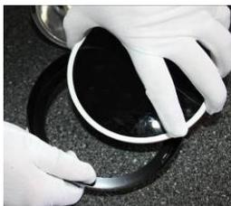
Fit the black filter glass back in the filter mounting ring.
