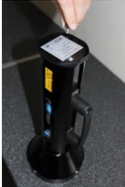
Place the Klercide UV Validation Torch on a solid flat surface. Unscrew and remove the thumb wheel on the rear of the torch.
