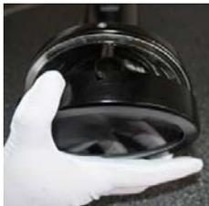
Replace filter mounting ring and black filter glass on the front of the torch and secure with the 4 x M4 screws and washers.
