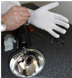
Put on lint free nylon gloves. This will avoid fingerprints contaminating the filter glass during reassembly.
