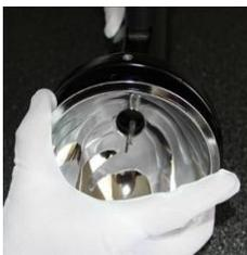
Put on lint free nylon gloves. This will avoid fingerprints which would burn into the quartz during operation and significantly reduce performance and UV bulb life.
