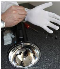
Put on lint free nylon gloves. This will avoid fingerprints contaminating the filter glass during reassembly.
